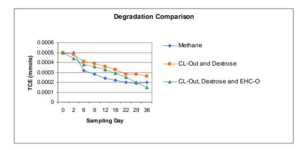
The microcosms were tested periodically for TCE and daughter product concentrations. The chart shows the average TCE concentrations in the three replicate microcosms. The untreated standards showed no degradation or removal of TCE and are not included in the comparison for simplicity. Daughter products, such as DCE or vinyl chloride were not detected in any of the microcosms, showing the TCE removal was complete.
